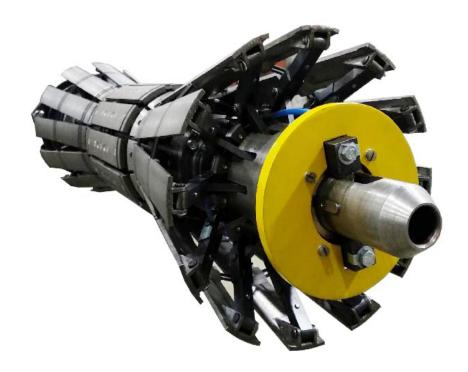
Assembly drum for radial tires is designed to assemble 6.50-10 inch tires for the SPK-8 machine.
