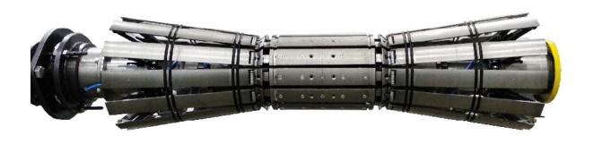
The wrapping of the tire cord plies onto the ring is carried out by free-rolling rollers placed on the segment.
